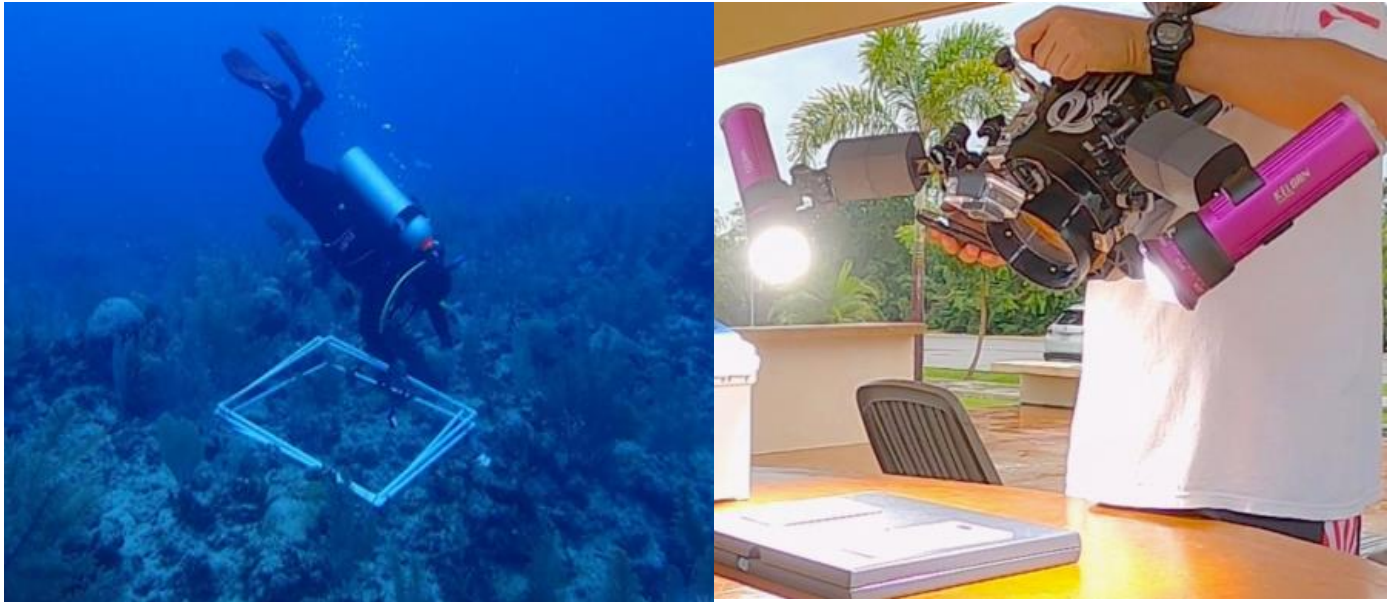
Figure 2. Left: the author collecting traditional data on juvenile corals during the dry season survey. Right: the MicaSense Red Edge-M short-range multispectral sensor adapted for underwater use.
