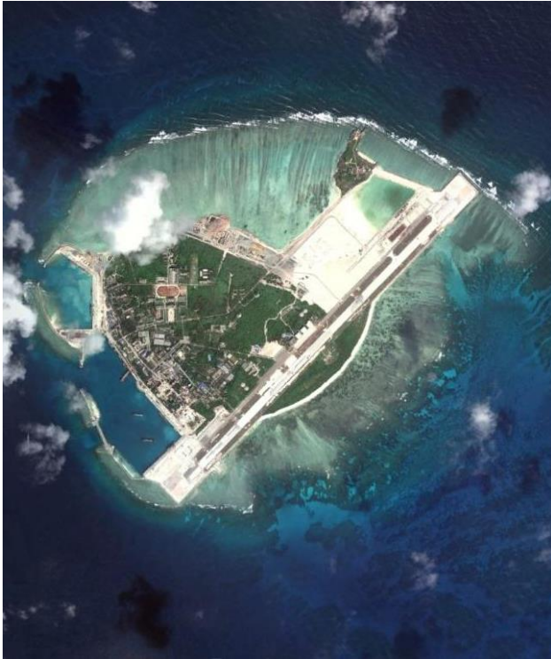
Figure 3. Filling to extend Woody Island in the Paracel group. Source: Google Earth 2016 (Google Earth and DigitalGlobe 2016).
