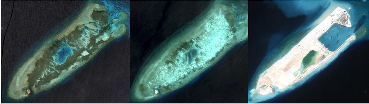
Satellite photos of Fiery Cross Reef: (left) 2006: small military outpost and largely healthy reefs, (middle) 2014: reef flat has been dug up for giant clams, (right) 2015 during artificial island construction, with plumes of sand and silt spreading onto the reef (a. CSIS Asia Maritime Transparency Initiative / Digitalglobe, b and c Google Earth/Digital Globe 2016).
