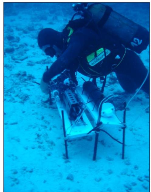
**Figure 3.** View of the data logger as set out on the reef to collect environmental parameters.
