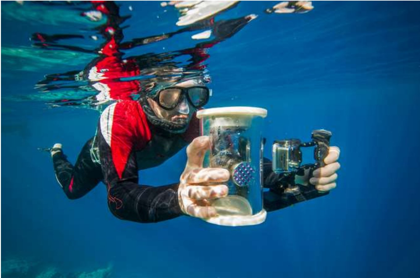
Figure 3. Customised tools for coral research. 3D printed UV torch container and camera stabiliser used for field coral imaging.
