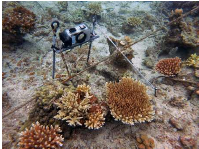
Figure 5 The camera arrangement used to monitor corals for spawning, taking a picture every 30 minutes.
