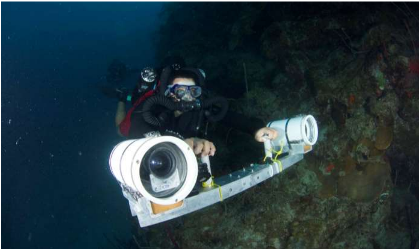
Figure 2. A CCR diver using a stereo-video system to conduct fish biomass surveys along reef transects. Post dive the footage from the two cameras are synchronized, allowing fish lengths to be accurately estimated. (Photo: Ally McDowell)
