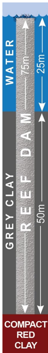
Figure 3. Section of reef dam.
