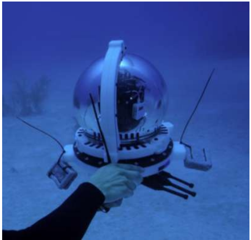
“Clean Sweep System” showing how the cleaning arm, just above the divers hand, wraps around the housing (Photo credit - courtesy Netflix / Chasing Coral).
