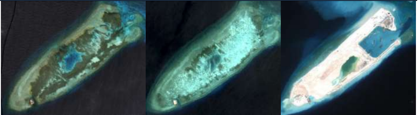
Satellite photos of Fiery Cross Reef: (left) 2006: small military outpost and largely healthy reefs, (middle) 2014: reef flat has been dug up for giant clams, (right) 2015 during artificial island construction, with plumes of sand and silt spreading onto the reef (a. CSIS Asia Maritime Transparency Initiative / Digitalglobe, b and c Google Earth/Digital Globe 2016).
