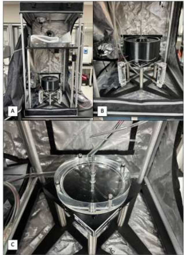
Figure 2. Example of a newly developed aquatic olfactometer. A) Overview of the entire olfactometer, B) Main testing instrument of the olfactometer. Choice arena is covered with a light blocking cover, and C) Choice arena covered with glass cylinder to create watertight seal within arena. Photo Credit: Clayton Vondriska.
